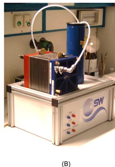
Fig. 7. (A) Performance curve of a 12 cell autonomous DMFC stack at different temperatures. Open symbols (full symbols) represent the stack voltage (power) vs. current density. (B) Image of the 12 cell autonomous DMFC system.
